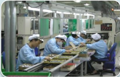
DIP ASSEMBLY LINE
